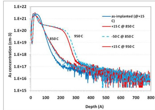
Figure 7: SIMS profiles of the As 2 keV  $1 \times 10^{15} \text{ cm}^{-2}$  implant after a 10s 850 °C and 950 °C RTP. Plotted are the as-implanted as well as the profiles for +15 °C and -50 °C implant temperature.
