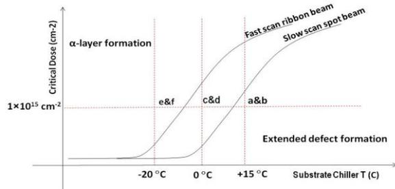
Figure 3: Cartoon illustrating the relationship between beam current density, implant dose and substrate T for a 6 keV  $1 \times 10^{15} \text{ cm}^{-2}$  carbon implant. Letters refer to the TEM pictures of fig. 2.
