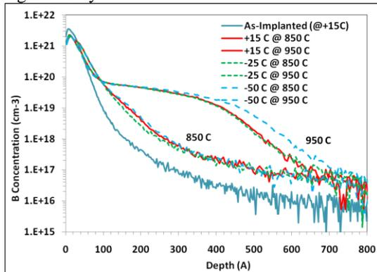
Figure 5: SIMS profiles of the B 300 eV  $1 \times 10^{15} \text{ cm}^{-2}$  implant after a 10s 850 C and 950 C RTP. Plotted are the as-implanted as well as the profiles for +15 °C, -25 °C and -50 °C implant temperature
