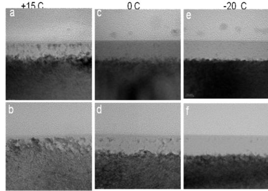
**Figure 2: HR-TEM data for a 6 keV  $1 \times 10^{15} \text{ cm}^{-2}$  carbon implant for a spot beam at low scan velocity (top row) and a ribbon beam at high scan velocity (bottom row) at three implant temperatures.**
