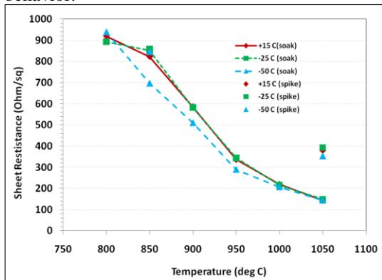
Figure 6: sheet resistance for As 2 keV  $1 \times 10^{15} \text{ cm}^{-2}$  at three different implant temperatures and after a 10s soak anneal between 800 °C and 1050 °C (lines+markers) as well as a spike anneal at 850 °C and 1050 °C (markers only).
