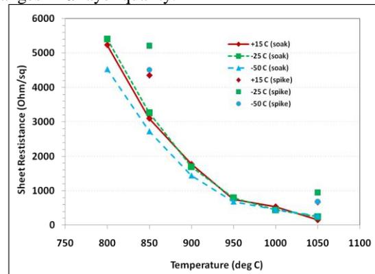
Figure 4: sheet resistance for B 300 eV  $1 \times 10^{15} \text{ cm}^{-2}$  at three different implant temperatures and after a 10s soak anneal between  $800 \text{ }^\circ\text{C}$  and  $1050 \text{ }^\circ\text{C}$  (lines+markers) as well as a spike anneal at  $850 \text{ }^\circ\text{C}$  and  $1050 \text{ }^\circ\text{C}$  (markers only).
