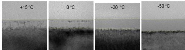
**Figure 1: HR-TEM data for a 6 keV  $1 \times 10^{15} \text{ cm}^{-2}$  carbon implant using a spot beam at different substrate chiller T between +15 °C and -50 °C.**
