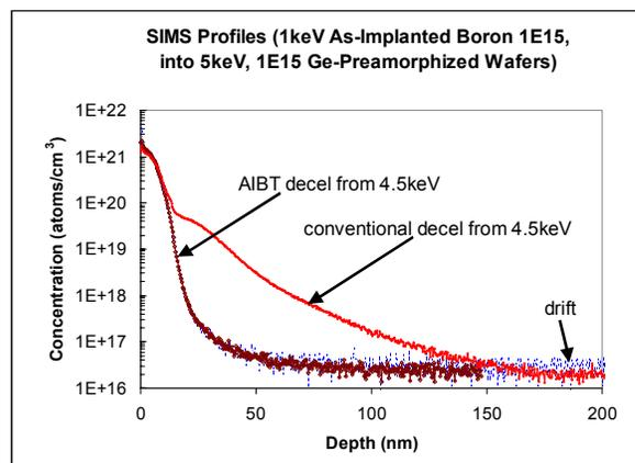
Figure 1. As-implanted SIMS profiles for 1keV  $B^+$ ,  $1 \times 10^{15}$  atoms/cm<sup>2</sup> implants on pre-amorphized wafers, using drift beam, conventional decel beam, and AIBT decel beam. The decel beams were decelerated from 4.5keV beams at  $5 \times 10^{-5}$  torr pressure in decel region.
