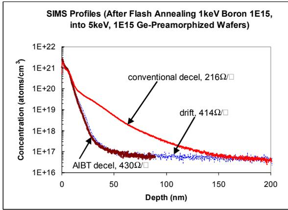
Figure 2. After-anneal SIMS profiles for 1keV B<sup>+</sup>, 1E15 atoms/cm<sup>2</sup> implants on pre-amorphized wafers, using drift beam, conventional decel beam, and AIBT decel beam. The decel beams were decelerated from 4.5keV beams at 5E-5 torr pressure in decel region.
