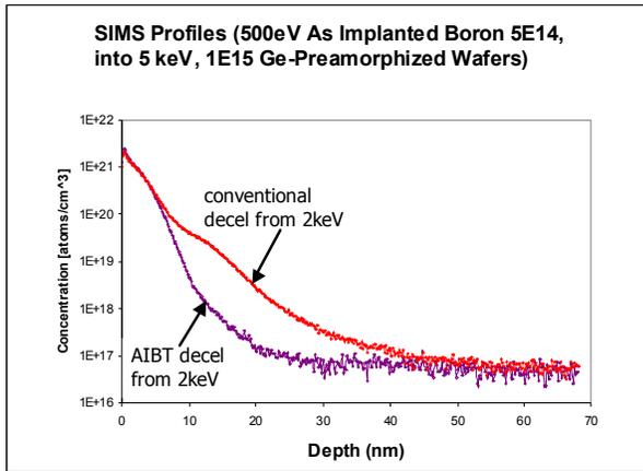
Figure 3. As-implanted SIMS profiles for 500eV B<sup>+</sup>, 5E14 atoms/cm<sup>2</sup> implants on pre-amorphized wafers, using conventional decel beam, and AIBT decel beam decelerated from 2keV beams.
