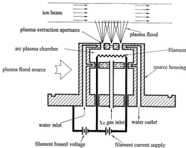
Figure 1. Functional block diagram of a plasma flood source.
