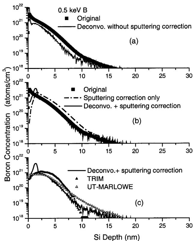
FIG. 3. Original SIMS boron profile, deconvoluted profiles, and simulated profiles. (a) Original SIMS profile and deconvoluted boron profile without sputtering correction, (b) original SIMS profile, deconvoluted profile with sputtering correction only, and profile with sputtering correction and deconvolution together, and (c) deconvoluted profile and simulated profiles from TRIM and UT-MARLOWE.
