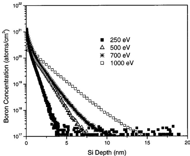
FIG. 1. SIMS profiles of boron measured at normal direction with oxygen flooding and incident oxygen beam at 250, 500, 700, and 1000 eV.
