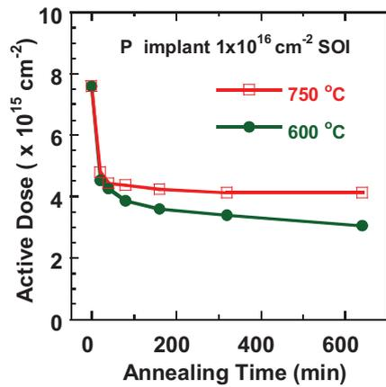
Fig. 5. Deactivation of phosphorus for samples implanted by phosphorus at a dose of  $1 \times 10^{16} \text{ cm}^{-2}$ .
