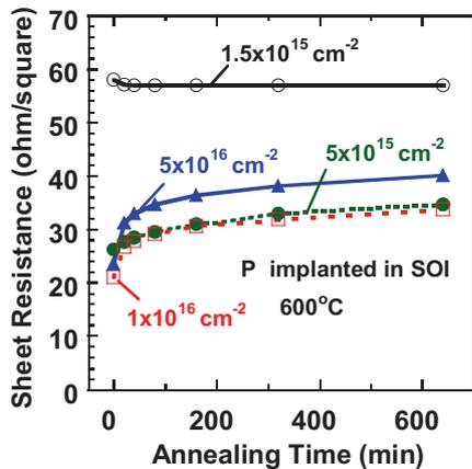
Fig. 2. Sheet resistance during deactivation at 600°C.
