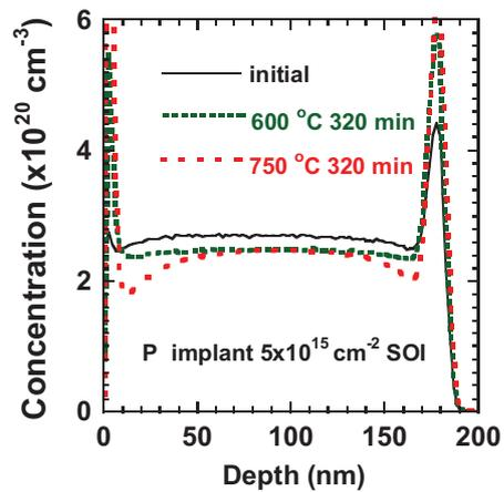
Fig. 6. SIMS profiles of phosphorus for samples with phosphorus implantation at a dose of  $5 \times 10^{15} \text{ cm}^{-2}$ .
