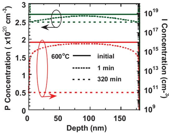
Fig. 8. Simulation for phosphorus and interstitial profiles at 600°C.
