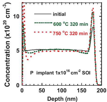
Fig. 7. Phosphorus SIMS profiles for samples implanted by phosphorus at a dose of  $1 \times 10^{16} \text{ cm}^{-2}$ .
