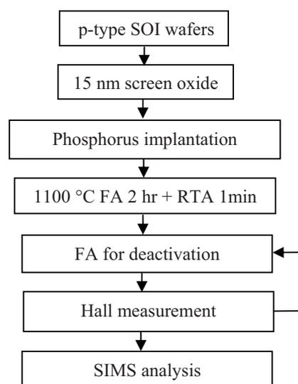
Fig. 1. Experimental procedure for this study.
