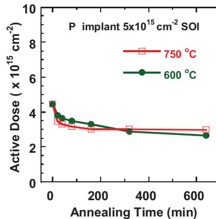
Fig. 4. Deactivation of phosphorus for samples with phosphorus implantation at a dose of  $5 \times 10^{15} \text{ cm}^{-2}$ .
