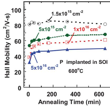
Fig. 3. Measured Hall mobility during deactivation at 600°C.
